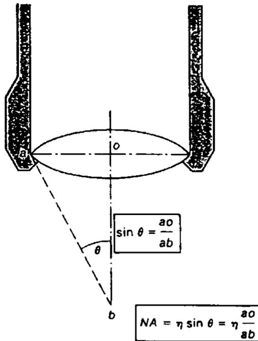
**Figure 2** A diagrammatic representation of numerical aperture. (NA).
